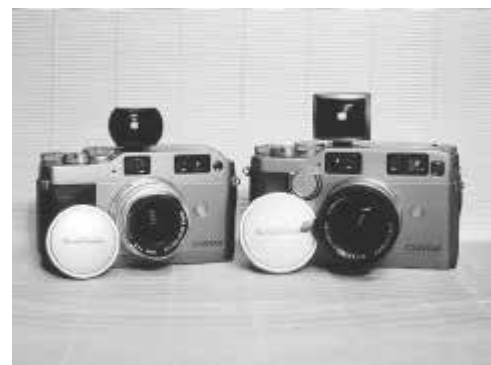
Zörk-Heliar lens conversions on Contax G1 and G2
